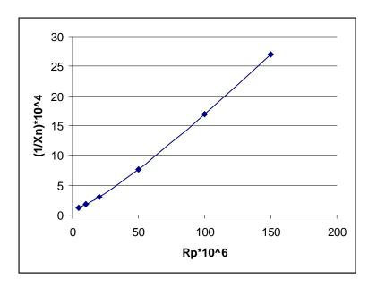
The plot is linear at low  $R_p$  (i.e., the first three points).  $C_M = \text{intercept} = 5.97*10^{-5}$ .
